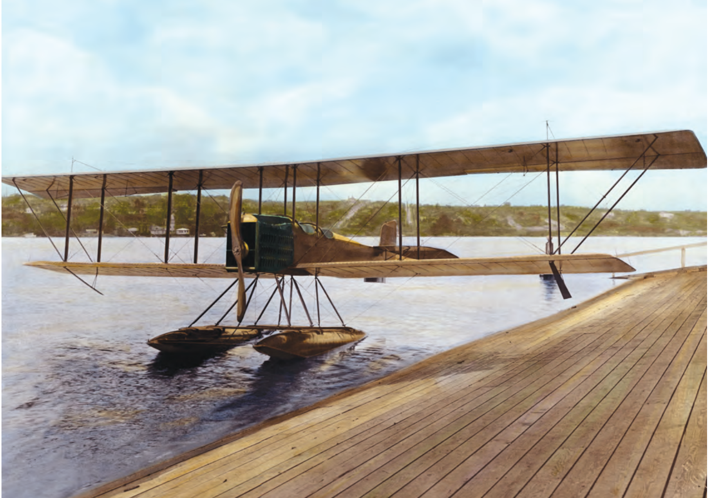
This idyllic photograph is taken of the B & W. It was the first Boeing product, named after the initials of its designers, William Boeing and Navy Lt. Conrad Westervelt. The first B & W, completed in June 1916, was made of wood, linen and wire. Similar to the Martin trainer that Boeing owned, the B & W had, among other improvements, better pontoons and a more powerful engine.
